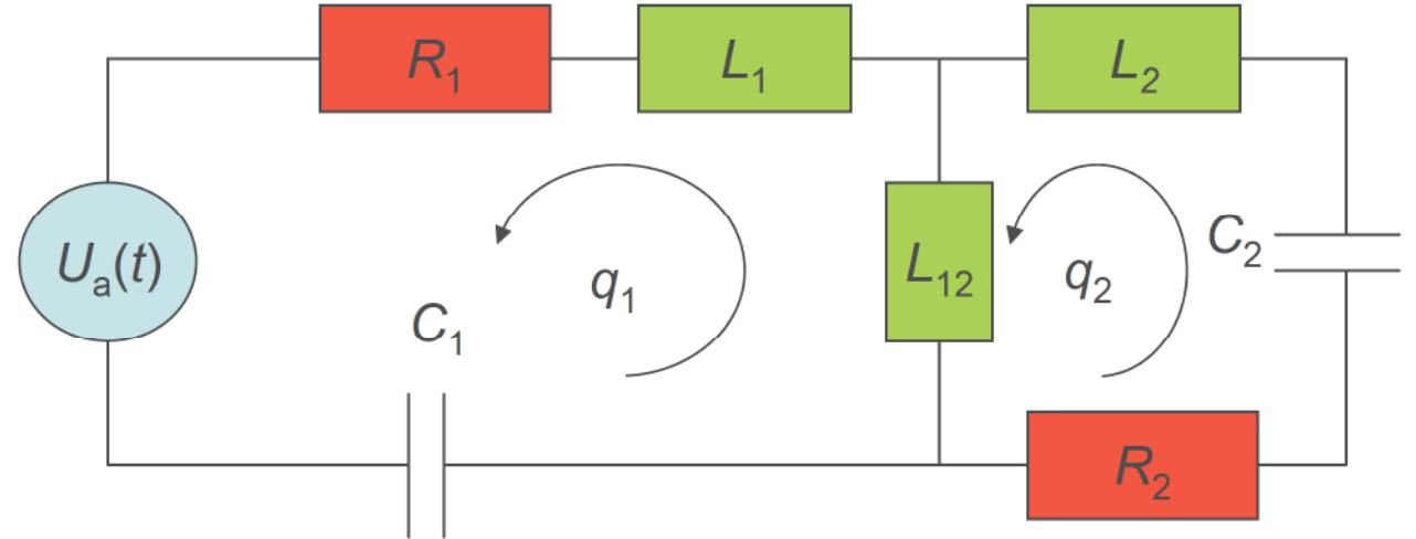
Assume  $q_1$  and  $q_2$  as the independent generalized coordinates, where  $q_1$  is the electric charge in the first loop and  $q_2$  is the electric charge in the second loop.
