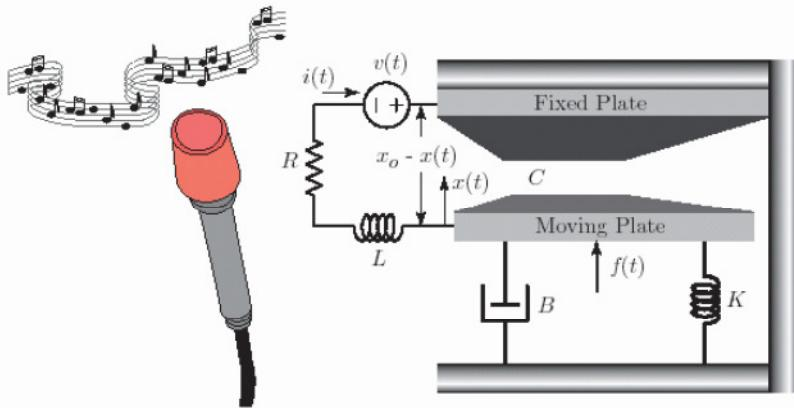
This system has two degrees of freedom (electrical and mechanical: charge  $q$  and displacement  $x$  from equilibrium)
